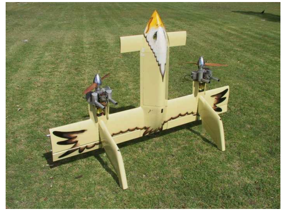
Fig. 3 – The T-Wing micro air vehicle flight tested by the University of Sidney (2002).
